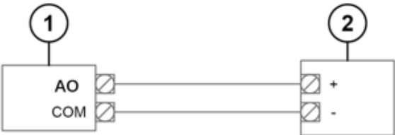
Figure 13: SM-8AO current or voltage output wiring
